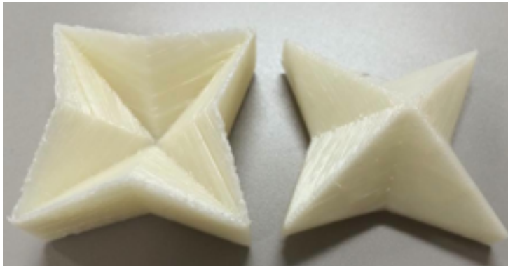
A set of folding mold for square tessellation pattern made by the 3D printer.
