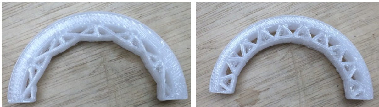
Fig 08. Second printing with adjusted parameters.
