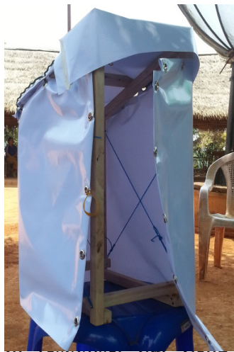
1:5 Model presented to Committee Materials: Water proof, Fire proof Vinyl Wooden frame with rope cross-bracing (hypothetical) Left: 1:5 Model Centre: Annabell Stubbs, Dr. Lynn Thiesmeyer Right: Interior shot
