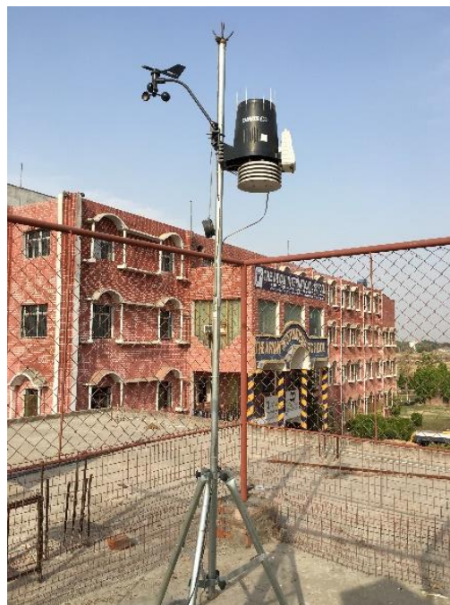
Figure 3. Automated weather station
