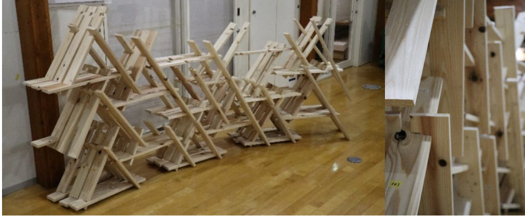
Timber Shelf Fabricated with CNC Milling: use of interlocking timber joints to create the self-standing curved structure
