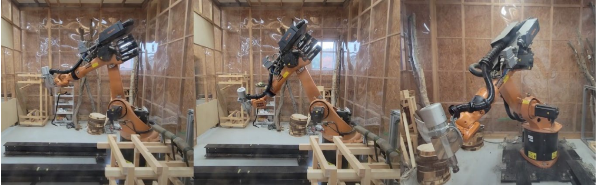
Offline Programming: Robot Following a Milling Path Defined by the Computer
