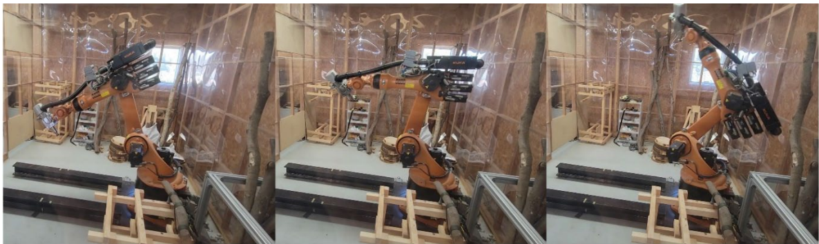
Real-Time Programming: Robot goes to the positions defined by the computer. The moment a location is selected on the computer, the robot reacts by going to that particular position.
